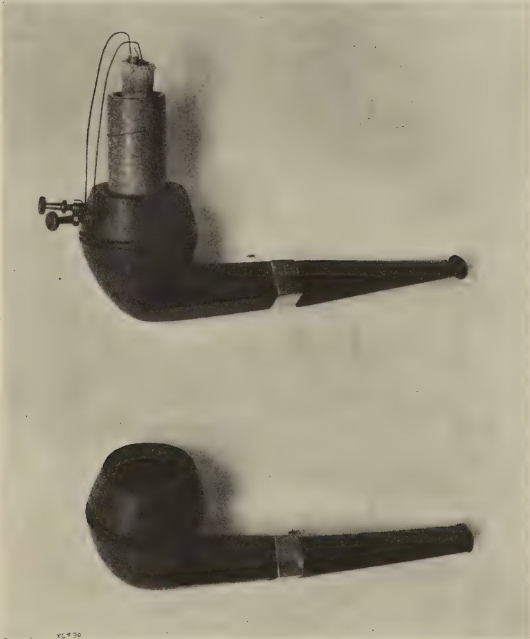
PLATE 2. The special experimental pipe (above) and the regular tobacco pipe (below). Note the exact similarity in form of the two pipes.
